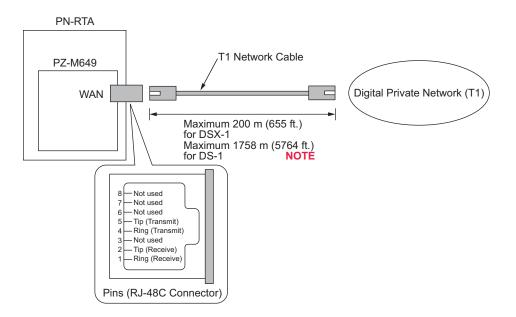
**NOTE:** The cable length can be set by the interface command via the CLI (T1 lbo short-haul FEET or T1 lbo long-haul DB). The default setting is short-haul 0 (0 to 40 m [0 to 132 ft.]). For details, refer to "Router Command Reference Manual".
